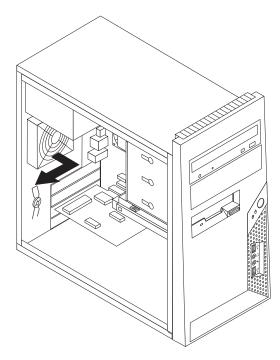
Figure 30. Removing the rear fan assembly
